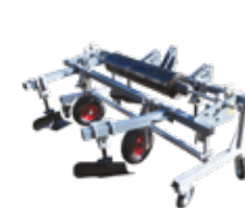
Mulch laying machine
